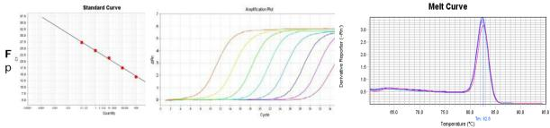
**Fig.9** The standard curve, amplification plot and melt curve of Vibrio alginolyticus quantitative polymerase chain reaction (qPCR). From down to up is Ref3, Ref4, Ref, Ref6, Ref7, Ref8; R2=0.998.
