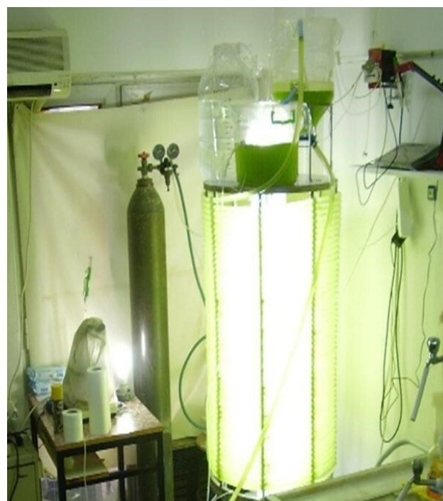
Figure 3. Helical Photobioreactor designed in the experiment 26
